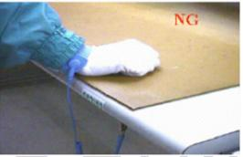
12.4 Please do not bend the film near the substrate glass.(this could cause film peeling and COF damage) and the peeling strength about 600g/cm, the bending <20times and the bending radius :R>0.8mm
